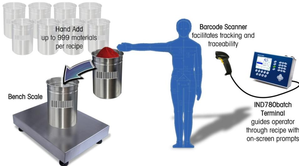
In this example you can see that the application involves the use of a single scale; the operator will be adding the materials to the scale by hand; a bar code reader will be used to scan each material before it is added to the scale; and the IND780batch terminal will guide the operator through each step of the recipe using its color HMI display.
